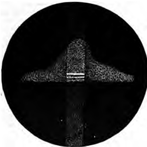
FIG. 92.—FLASH SPECTRUM OF SODIUM PRODUCED BY ANOMALOUS DISPERSION.
