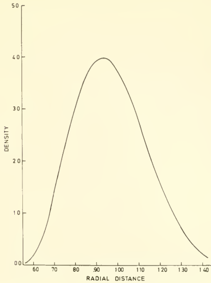
Figure 2.—Particle density in the stream along a radius vector in the symmetry plane of the stream, case I; arbitrary units.
