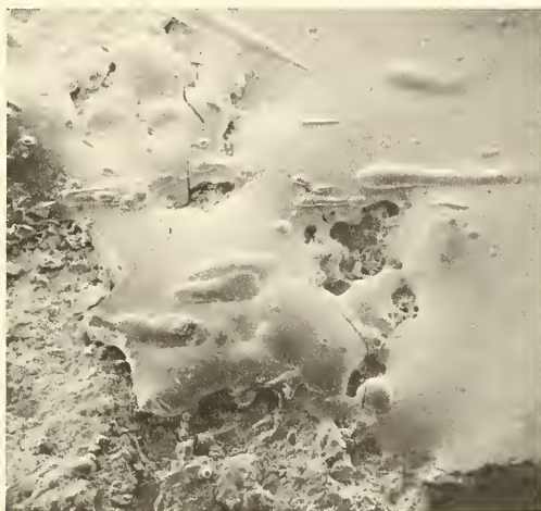
Figure 6.—Glass splash over friable breccia (rock 12017) from Oceanus Procellarum. Scanning electron micrograph taken at a magnification of \times 50 .
