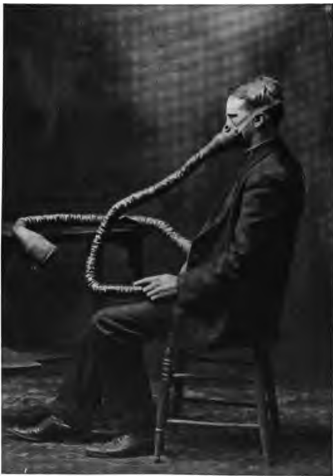
FIG. 71.—A DEVICE FOR THE REMOVAL OF THE RESPIRATORY PRODUCTS FROM THE RESPIRATION CHAMBERS. (SIDE VIEW.)
