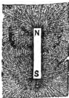
FIG. 51. IRON FILINGS ON PAPER OVER BAR MAGNET, SHOWING MAGNETIC FIELD AND LINES OF FORCE.
