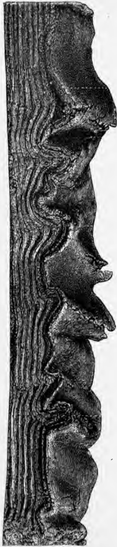
Figure copied from Nature , Vol. XIX, p. 104, illustrating Professor A. Favre's experiment upon the compression of a layer of clay.
