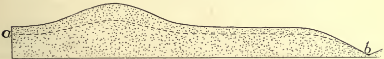
FIG. 79.—Diagram illustrating the position of the ground-water surface (the dotted line) in a region of undulating topography.
