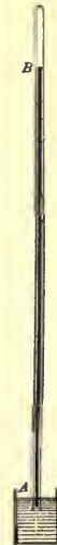
FIG. 577. — Diagram to illustrate the principle of the barometer. The pressure of the air at A maintains the mercury at l in the tube when there is no air in the tube above B.
