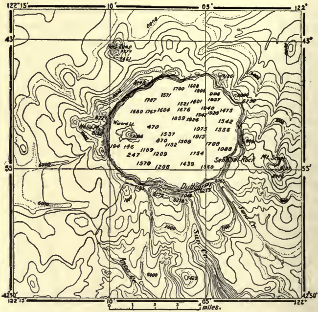
FIG. 333.—Map of Crater Lake, Ore. Contour interval 200 feet. Soundings in feet. Lake surface 6239 feet above the sea-level. (U. S. Geol. Surv.)
