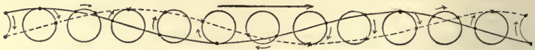
FIG. 340.—Diagram to illustrate the movement of water in waves. The small circles represent the movement of water particles.
