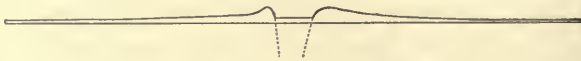
FIG. 194.—Levees of the Mississippi in cross-section, four miles north of Donaldsonville, La. Vertical scale \times 50 . The horizontal line represents sea-level. The bottom of the channel is far below sea-level at this point.
