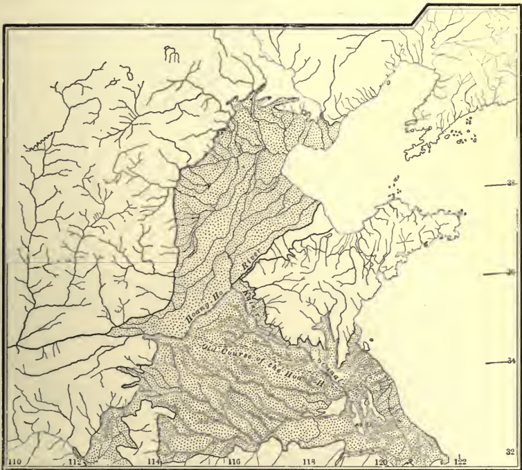
FIG. 207.—Diagram illustrating changes in the course of the Yellow River. The shaded area represents the area subject to flooding by the main stream and its tributaries. (Richthofen.)
