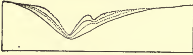
FIG. 134.—Diagram illustrating how one gully takes another as a result of lateral erosion.
