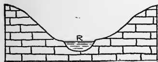
FIG. 147.—A deeper and narrower channel than that shown in Fig. 146, with the same gradient. A stream in a channel such as is represented in Fig. 147 will flow faster than one in such a channel as that shown in Fig. 146.
