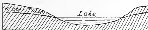
FIG. 330.—If the water table about a lake is above the lake level, there will be no leakage from the lake, even if its basin be of porous material.
