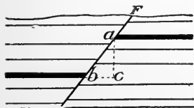
FIG. 428.—Diagram of a normal fault.
