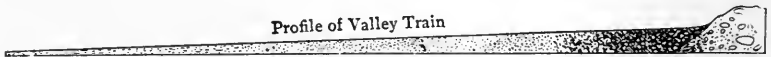
FIG. 299.—Diagram to illustrate the profile of a valley train, and its relations to the terminal moraine in which it heads.
