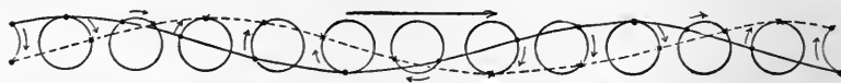
FIG. 340.—Diagram to illustrate the movement of water in waves. The small circles represent the movement of water particles.
