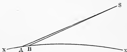
FIG. 524.—Diagram to illustrate the way in which a degree of latitude is measured. When the observer has traveled so far along the surface that the position of the pole-star has changed 1^\circ , the distance between the two stations, A and B , is a degree.
