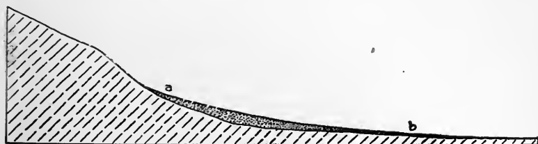
FIG. 210.—Diagrammatic profile and section of an alluvial fan.
