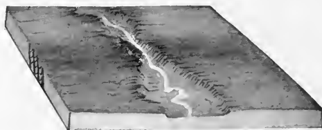
FIG. 168.—Diagram showing a narrow place in a valley where the stream crosses a hard layer of rock.
