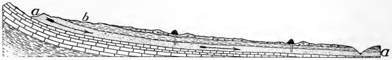
FIG. 77.—Diagram showing how water falling in one place may flow underground to another and there be brought to the surface. The layer a is porous and water entering it in the mountains follows it to the plains.
