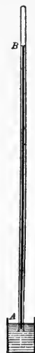
FIG. 577.—Diagram to illustrate the principle of the barometer. The pressure of the air at A maintains the mercury at B in the tube when there is no air in the tube above B.
