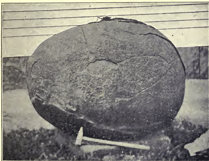
FIG. 90.—OVOIDAL BLOCK OF GRANITE Produced by weathering. Redstone Quarry, Westerly, R. I. From U. S. Geological Survey.
