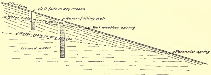
FIG. 124.—WATER TABLE, WELLS, AND SPRINGS
