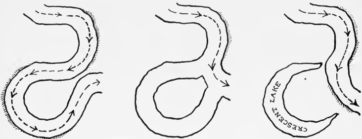
FIG. 149.—HOW CUT-OFF AND OXBOW LAKES ARE FORMED
