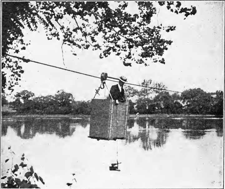
FIG. 135.—MAN MEASURING STREAM FLOW
