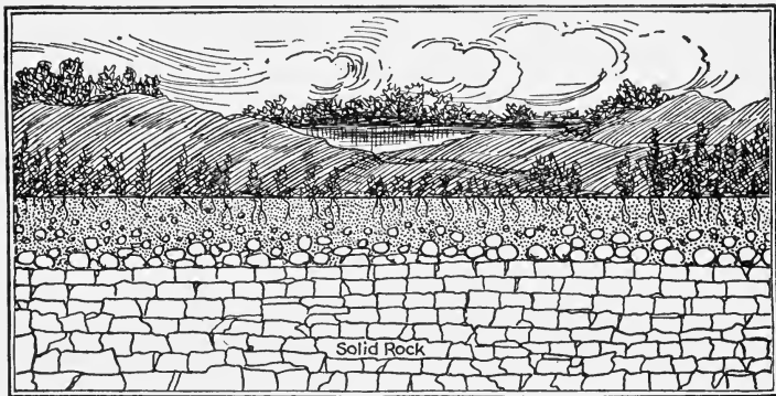
FIG. 98.—DIAGRAM OF RESIDUAL MANTLE ROCK
