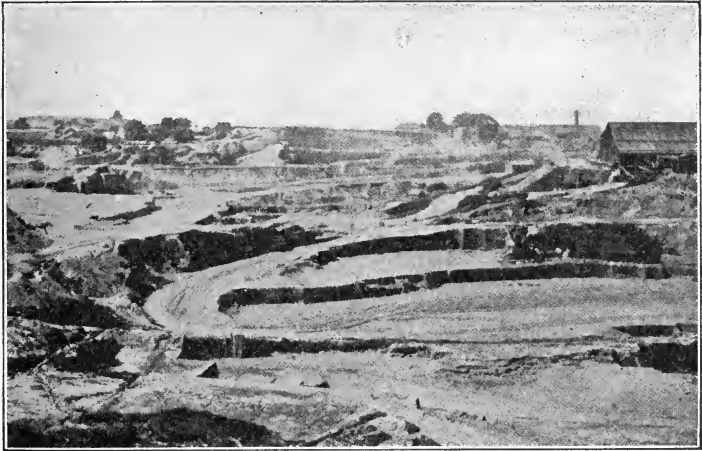
FIG. 104.—STRATIFIED CLAY (HAVERSTRAW, N. Y.) Used chiefly for bricks.
