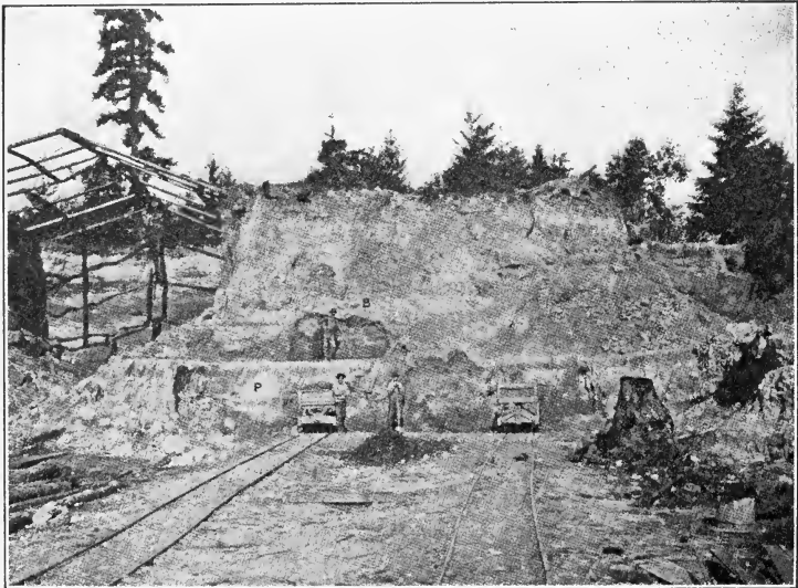
FIG. 105.—CLAY PIT (NEAR VANCOUVER, WASH.) B, gray brick loam. P, blue clay used for terra cotta.
