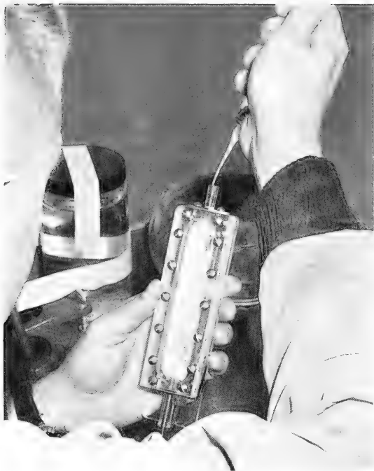
Figure A2. Scholander analyzer for dissolved gases. The capillary shown inside the lucite water jacket is calibrated in 100 divisions equivalent to a total volume in this case of slightly less than 30 cubic millimeters. The threaded plunger partly shown at bottom permits precise control of the gas bubble and liquid absorbents within the capillary.
