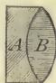
FIG. 57.—Achromatic lens. A, Plano-concave lens of flint-glass; B, biconvex lens of crown-glass.
