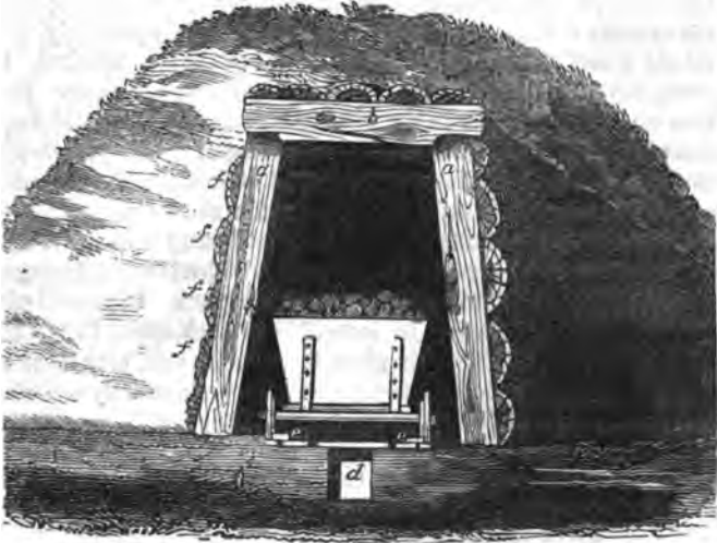
FIG. 56.—VIEW OF THE TIMBER OF A DRIFT OR COAL MINE.
