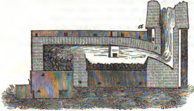
VIEW OF THE INTERIOR OF A PUDDLING FURNACE.
