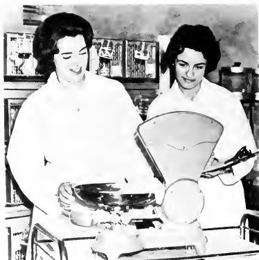
Home Economics Students test fading scientifically with a clothing fadometer.
