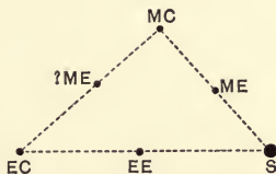
FIG. 29.— S represents the sun; EC , the centre of the earth's orbit, to be placed as best suited; MC , the same for Mars; EE , the earth's equant, or point about which the earth uniformly revolved ( i.e. the point determining the law of speed about the sun), likewise to be placed anywhere, but supposed to be in the line joining S to EC ; ME , the same thing for Mars; with ?ME for an alternative hypothesis that perhaps Mars' equant was on line joining EC with MC .
