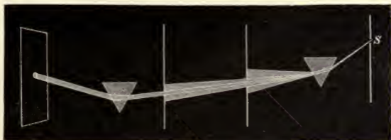
FIG. 64.—A single constituent of white light, obtained by the use of perforated screens is capable of no more dispersion.
