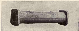
Cast Iron Pipe 160 Years Old—From Line Laid in Clermont-Ferrand, France. Still in Regular Service
