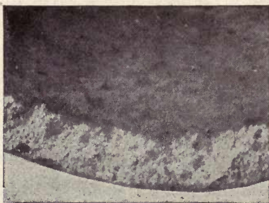
Fig. 5—Effect of Rust on Cast Iron
