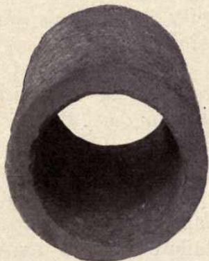
Section of Cast Iron Water Pipe in Philadelphia 98 Years Old
