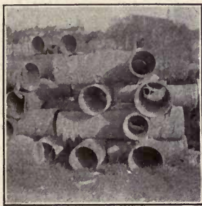
Burlap and Tar Coated Steel Pipe. Coating Melted by the Sun and Running Off in Sheets.
