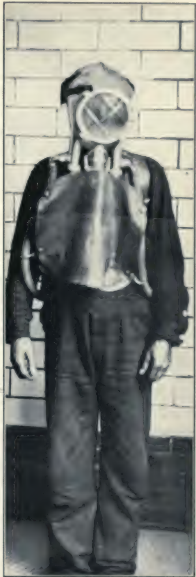
PLATES 19 AND 20.—WORKMAN EQUIPPED WITH SAFETY HOOD, READY TO ENTER A GASEOUS ATMOSPHERE
