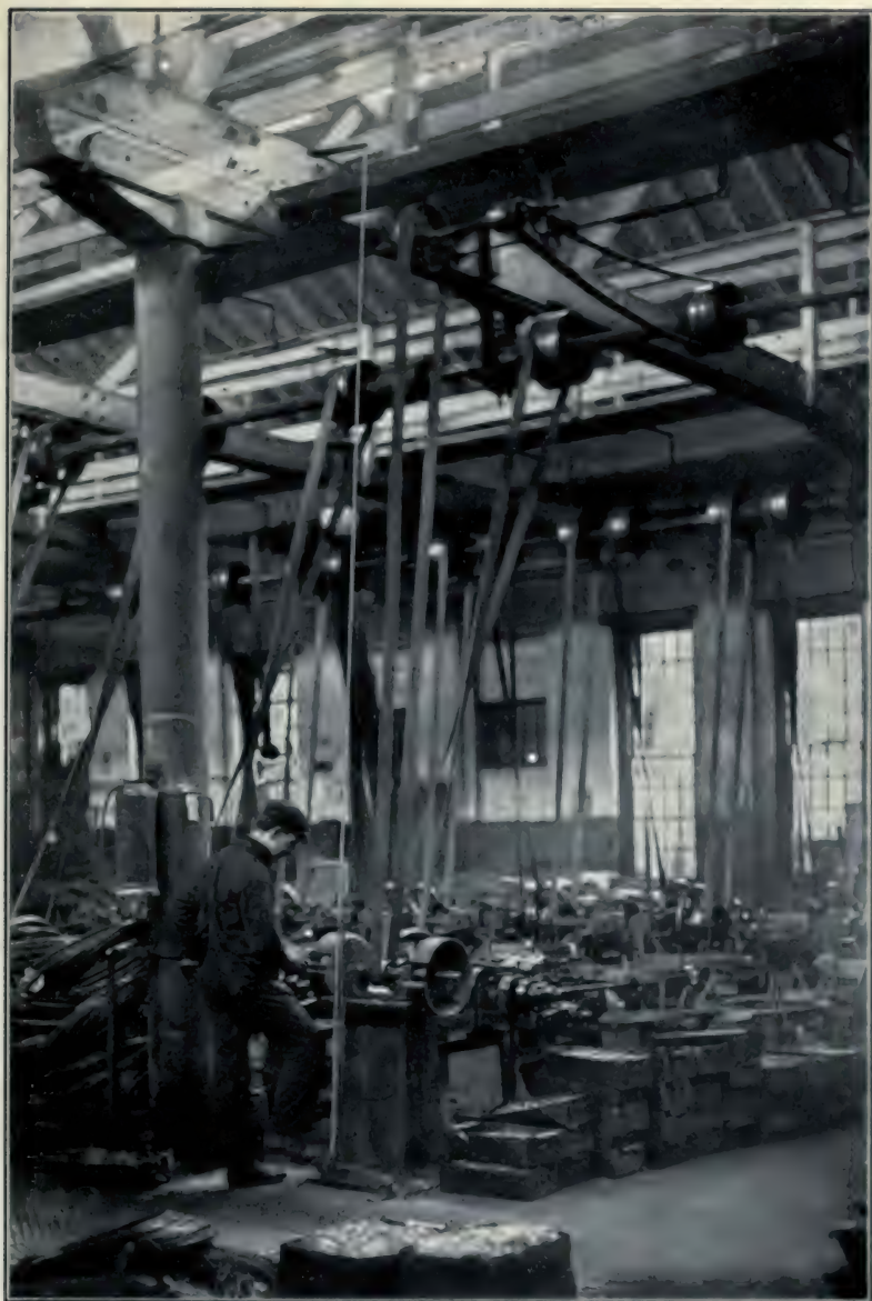
PLATE 11.—VIEW IN NAIL MILL SHOWING SAFETY HOODS OVER EMERY GRINDERS, WHICH ARE FLANGED OUT OF A SOLID PIECE OF STEEL PLATE
