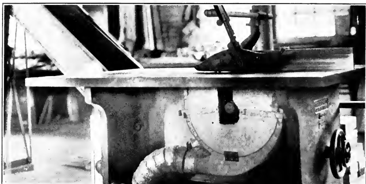
EXHAUST TUBINGS SUCKING DUST FROM A CIRCULAR SAW
