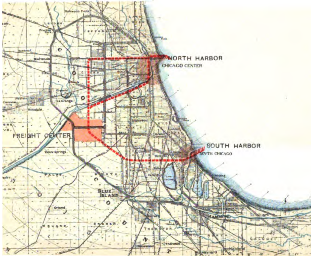
LXIX. CHICAGO. DIAGRAM OF A SYSTEM OF FREIGHT HANDLING FOR LAND AND WATER TRANSPORTATION, TO BE WORKED IN CONJUNCTION WITH ONE ANOTHER. (1) A central clearing and warehousing yard. (2) A north harbor at the mouth of the Chicago River. (3) A south harbor at the mouth of the Calumet River. (4) Underground freight lines interconnecting the city stations, the central yard, and the two harbors; these lines are shown in red; they do not represent exact locations of the routes.
