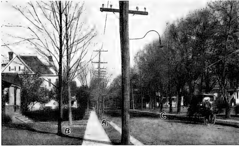
Fig. 14. Trees on curb, A, must compete with electric wires. Those inside walk, B, have head-room. Note fine row, C, protected from street by sidewalk.
