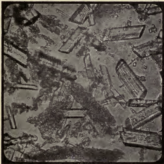
No. 7. Transformation of gypsum, "overburnt" at a temperature of 600-700 centigrade, into crystals of di-hydrate by means of alum solution. To be compared with No. 1. Magnified 360 times.
