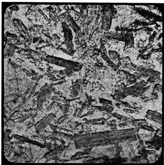
No. 8. Slow-setting plaster. Micro-photograph taken from van't Hoff's and Just's publication. By them believed to be hydraulic gypsum or floor-gypsum.
