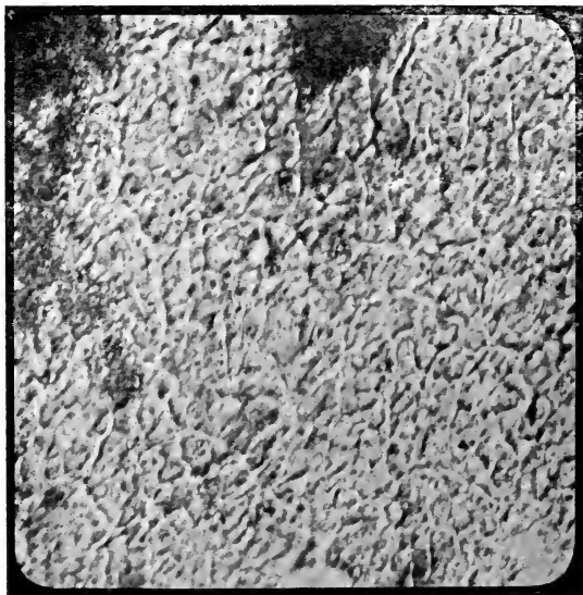
No. 13. Hydraulic gypsum burnt at 900 centigrade. Section through an unbroken piece showing the granular elements composing it in their original place. Magnified 750 times.
