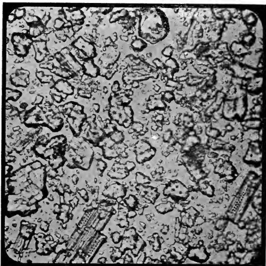
No. 10. Grains composing hydraulic gypsum. Same preparation as No. 9. Magnified 360 times.
