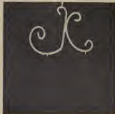
Articles that have been dip-coated frequently acquire tear drops that won't drain from their lower edges prior to drying, as illustrated here.
