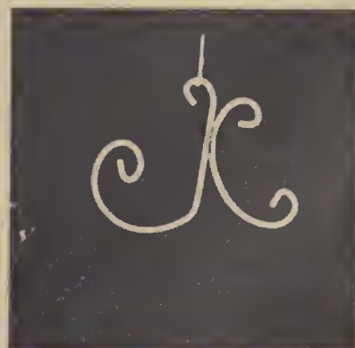
As shown here, a dip-coated article can be dried or cured after it has been electrostatically "detered" without unsightly blisters due to the presence of excess coating materials.
