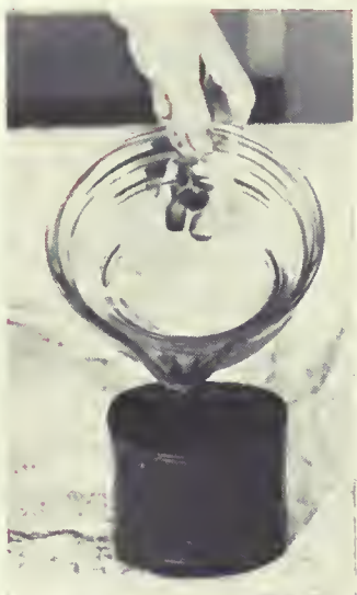
A water-clear polyester resin is poured into a flexible bleed mold, wherein Silicone exudations will serve as parting agents for the cured polyester cast.
