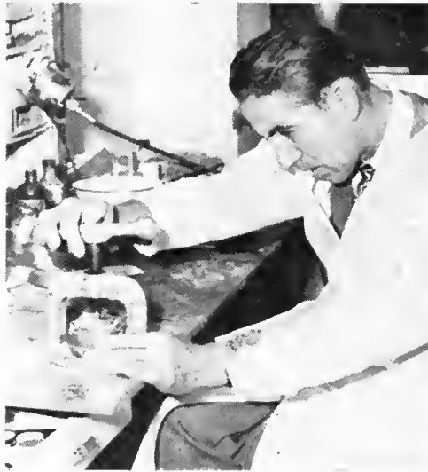
A bench clamp is used to prepare a squeeze mold for the casting and water-curing of acrylic resins.
