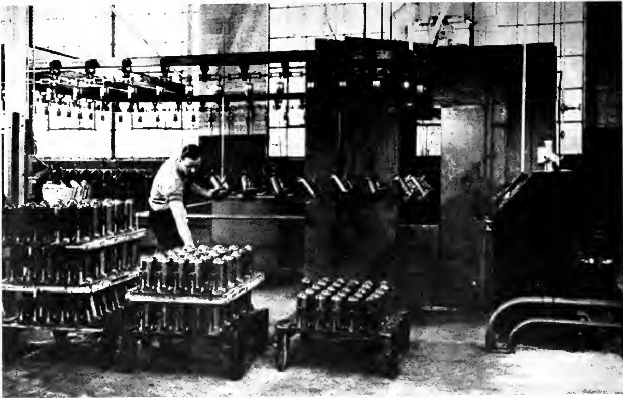
As pictured here, a single worker can maintain high-speed production when products are finished with electrostatic spray equipment.
