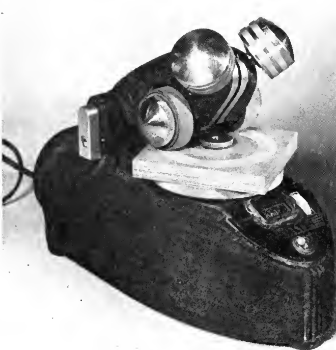
Figure 3. Taber abraser with typical modified-wood specimen in test position. (CS-17F calibrase wheels and 1,000 gram loads.)
