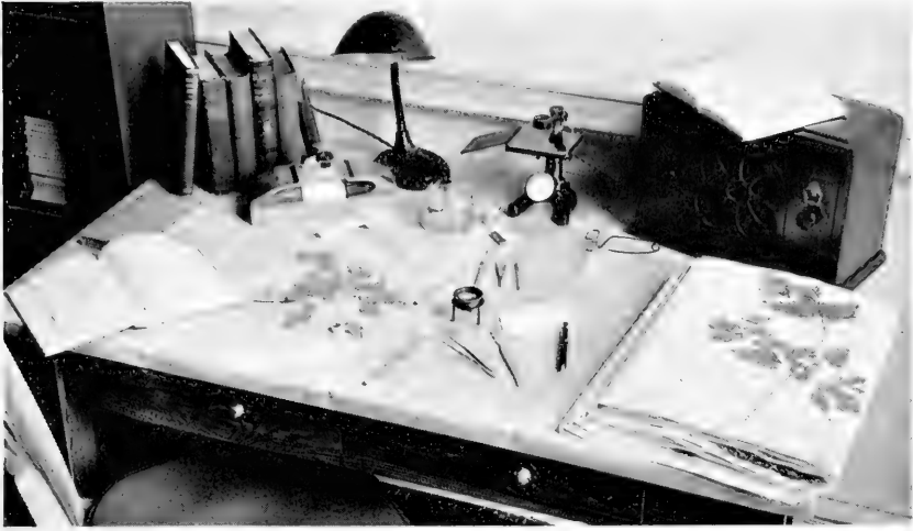
FIG. 5.—Equipment on a botanizer's work table. The articles on the table include dissecting needles, forceps, a scalpel, a ruler, watchglasses, test tubes and test tube holders, an alcohol lamp, a tripod magnifier and two dissecting microscopes.
