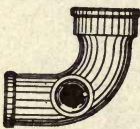
Fig. 181. Quarter-Bend with Side "Outlet."
