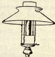
Fig. 112. Mantle Burner with Chimney and Shade.
