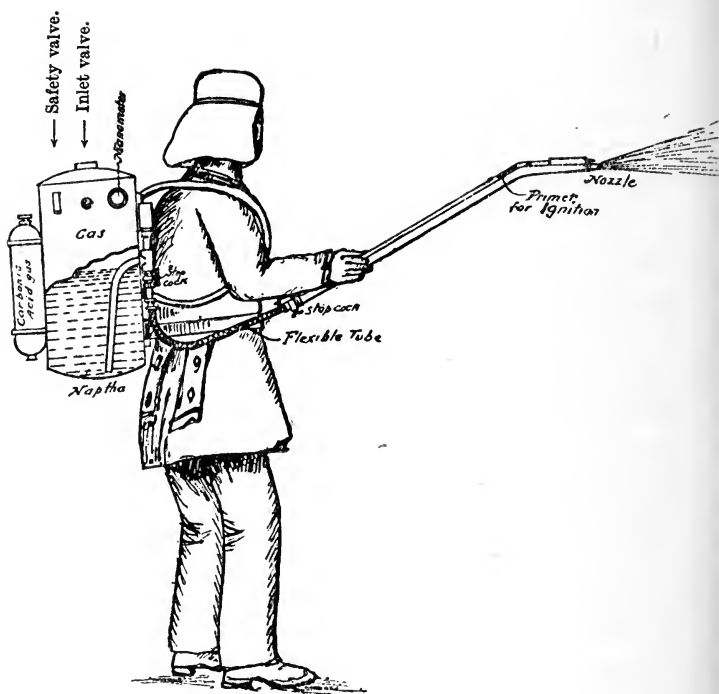
FIG. 9. The "liquid-fire" spray.
