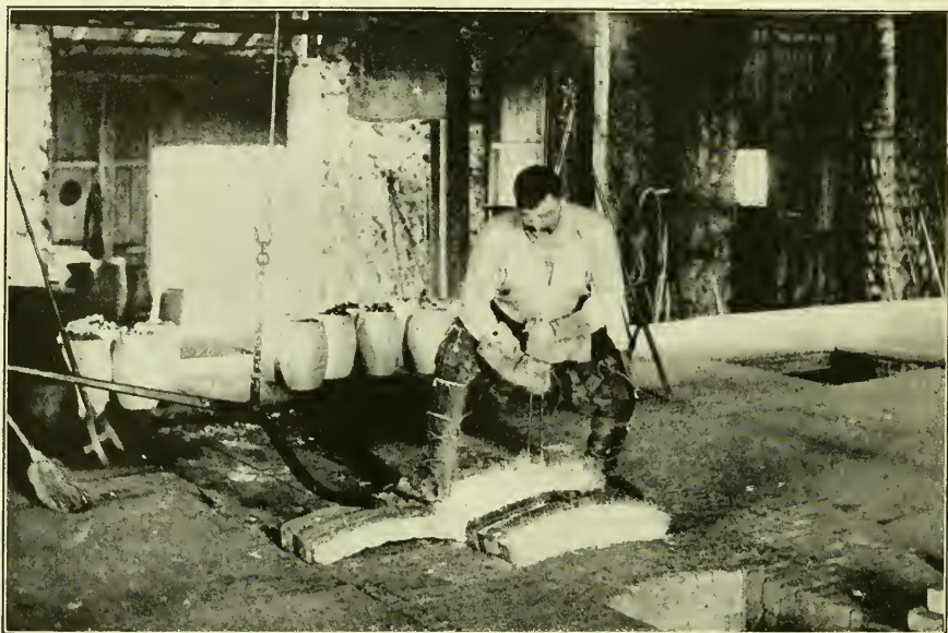
PULLING A POT IN A CRUCIBLE STEEL PLANT.
