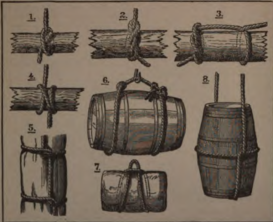
Commonly Used Hoisting Hitches.
