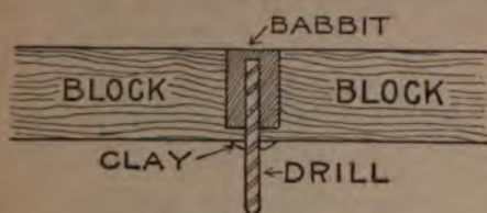
Repairing the Drill
