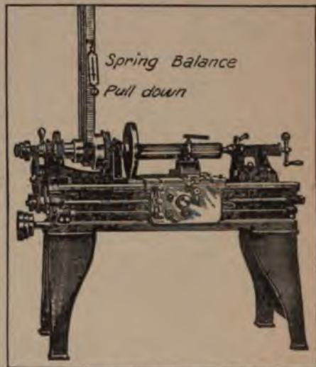
To Obtain the Horsepower of a Lathe
