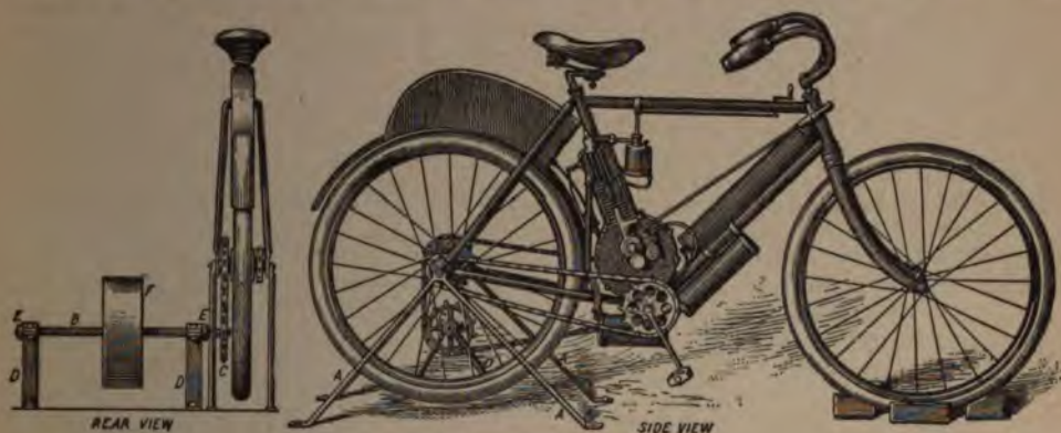
Using a Motorcycle for Shop Power
