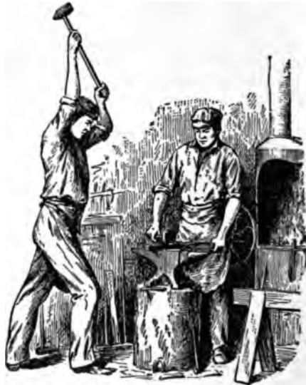
Fig. 4. The Force of the Blow Depends on How the Sledge is Grasped
