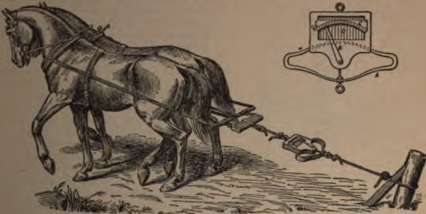
Fig. 5. Testing a Team by Means of a Dynamometer.
