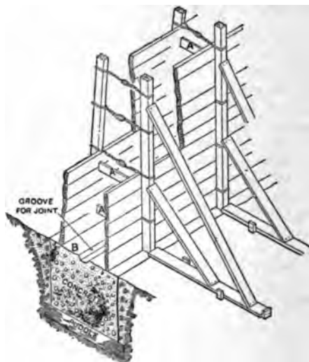
Form for Concrete Work
