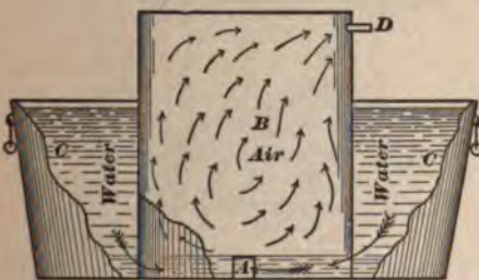
Emergency Air Compressor
