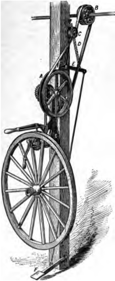
Attaching Power to a Tire Bolter.
