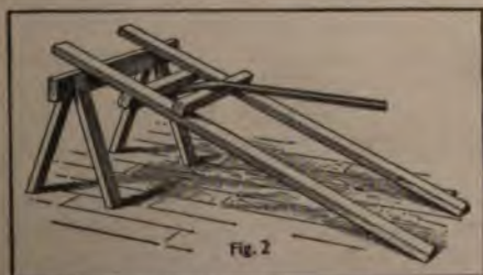
To Bend 2-in. Pipe and Up
