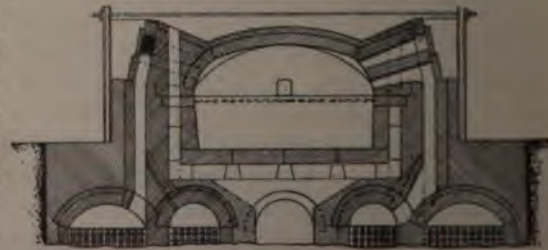
SIEMENS TANK FURNACE. Transverse section.
