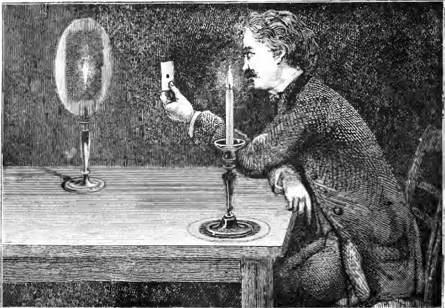
IMAGE FORMED BY A HOLE IN A CARD.
