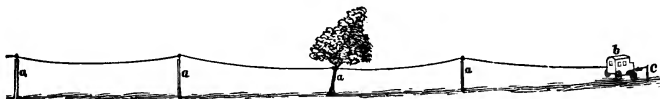
THE FIELD TELEGRAPH.— a a a , line-wire supported on posts and tree; b , station-wagon; c , earth-conductor.
