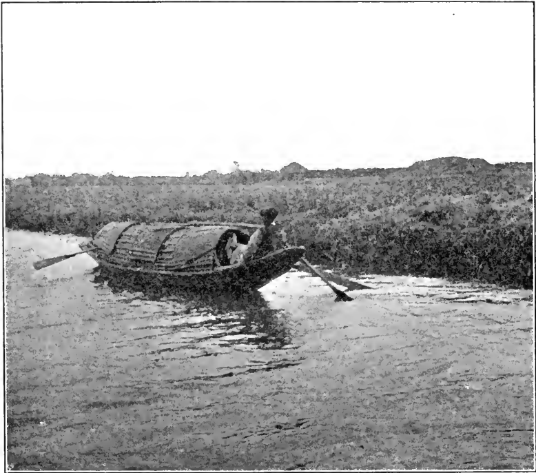
FOOT-BEAT, A FAST PASSENGER CRAFT ON CANALS IN YANGTSE DELTA. THE SIDE OAR IS BEING OPERATED BY THE FEET.
