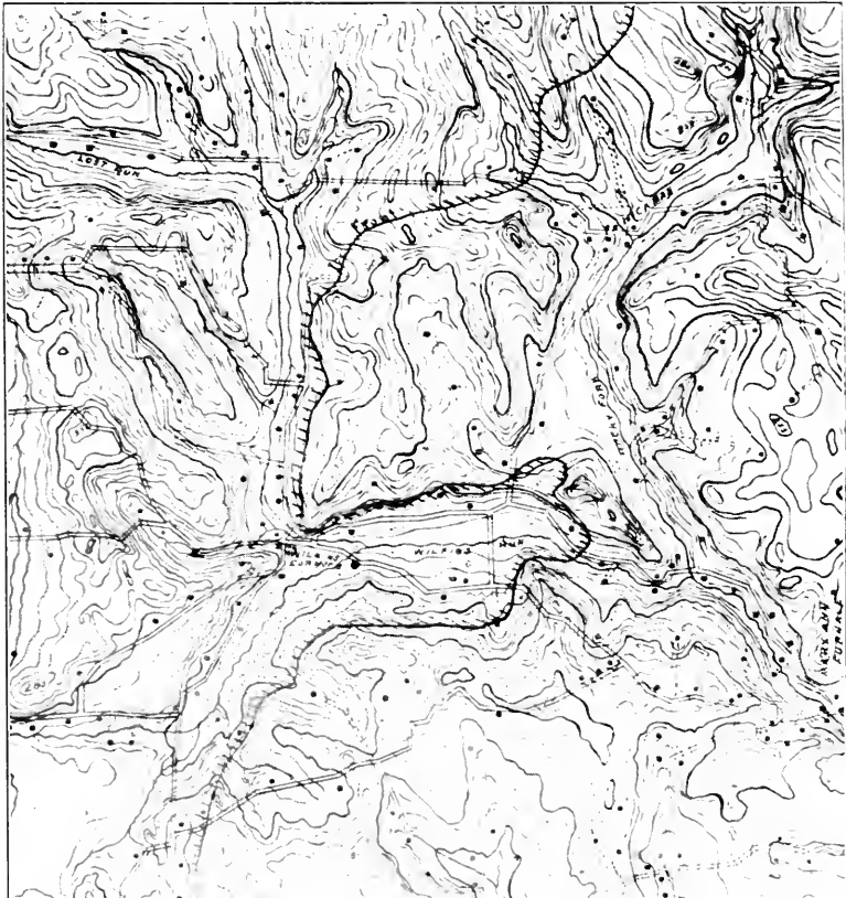
A RECONNAISSANCE CONTOUR MAP in which the altitudes were ascertained by working aneroids in pairs, a method explained in the Journal of Geology , Vol. XV. (1907), p. 492. In this area there are 203 dwellings, 148 of which are located at springs.
