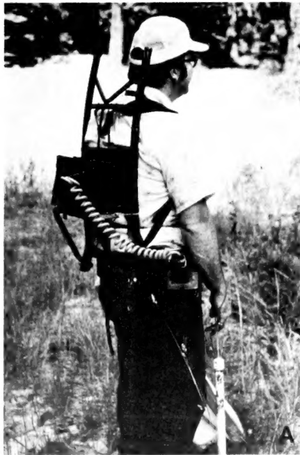
Figure 2.--(A) Pack-frame with mounted battery and side holster for vacuum; (B) collecting arthropods from beating cloth.
