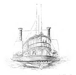
from this to an American river steamer is like that from an Oriental temple to a Lancashire factory. In the river steamer the hull is reduced to the position of an almost invisible carrier, and a huge deck-house covers everything. The arrangement is convenient, but it is both ugly and dangerous, as some accidents have proved. This is the extreme of the big deckhouse. The other extreme, that of the small one, is
