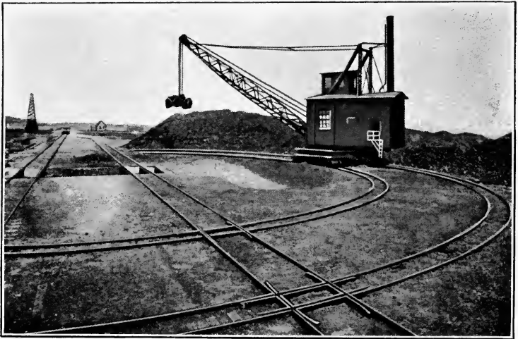
STEAM CRANE FOR CIRCULAR COAL STORAGE SYSTEM (20 ft. gauge, 80 ft. radius, 2 ton bucket, 80,000 tons storage capacity).
