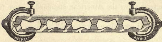
Fig. 80, Gang Mold, Screw Clamp.
