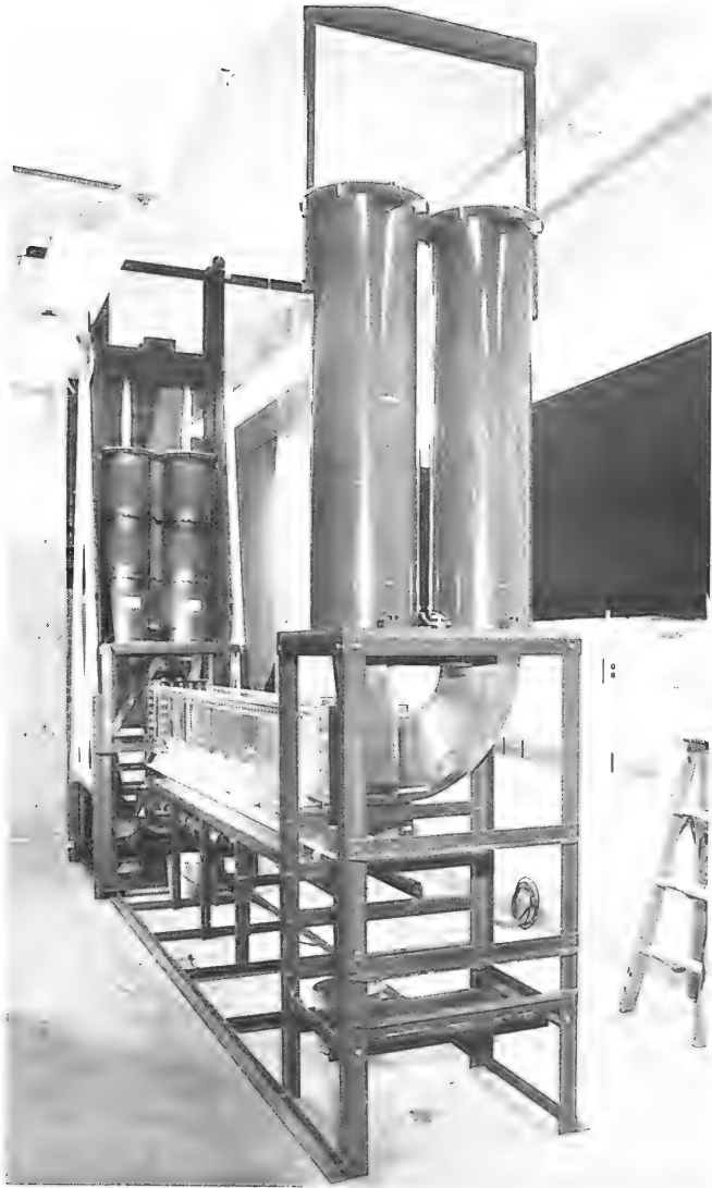
Figure 2. Photo of the tunnel from the reservoir end.
