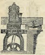
Vertical Saw Frames, for Cutting Log Timber, all sizes.
