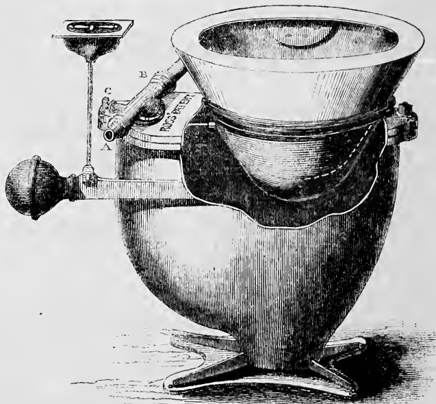
Fig. 1.—The ordinary Pan Water-Closet, with part of Trunk broken, to show mode of Working Valve.
