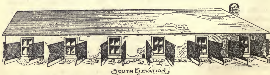
Fig. 32. Brooder House with Incubator Cellar,—Main house, 16 x 52 ft.; wing, 8 x 16 ft.; basement, 16 x 16 ft.; hall, 4 ft. wide; pipes 8 in. from the floor, six one-inch flow pipes; one two-inch return pipe. House double boarded with paper between. Cost complete, about $250.
