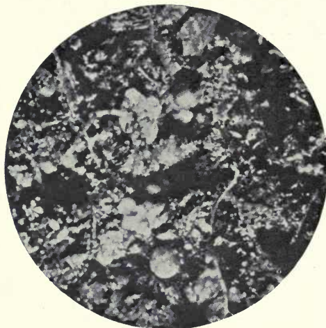
Fig. 114a.—Micro-photograph of soot, ash, cinders and mineral debris emitted from smoke stack of a boiler burning coal on grates or in retorts.
