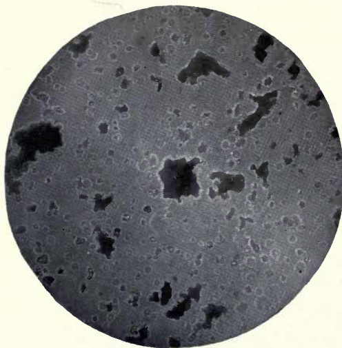
Fig. 114.—Micro-photograph of ash from pulverized coal collected in chamber of stationary boiler.
