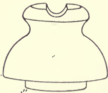
HEIGHT 3\frac{1}{4} " TESTED AT 40,000V.
