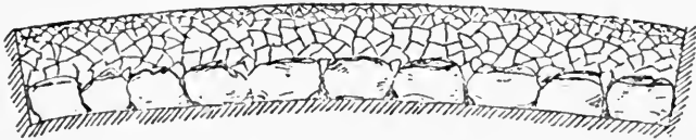
Fig. 86.—A Telford road.
