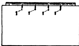
Fig. 58—English style of lacing boards.
