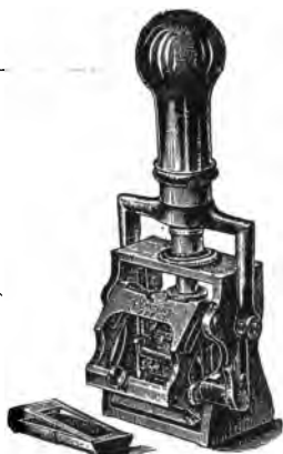
Fig 120—Hand numbering machine.
