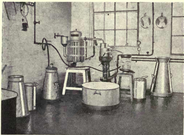
SMALL DAIRY, SHOWING TURBINE DRIVEN PASTEURIZER AND SEPARATOR.—MILK FED INTO PASTEURIZER FROM TANK ON RECEIVING PLATFORM OUTSIDE.
