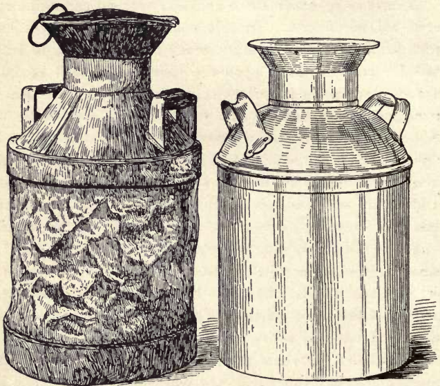
FIG. 55—RESULTS OF THE ROUGH USAGE ON THE RAILROAD It is almost impossible to clean the can on the left
