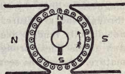
Figure 52 Armature reaction in a dynamo.
