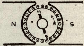
Figure 53 Counter magnetic motive force of armature reaction.
