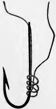
FIG. 12. FINISH-OFF OF WHIPPING.
