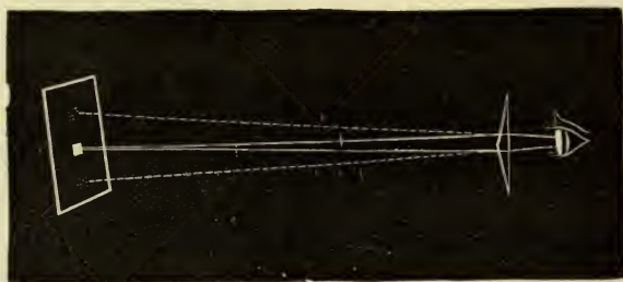
FIG. 74.—Maddox's double prism, illustrating the three images.
