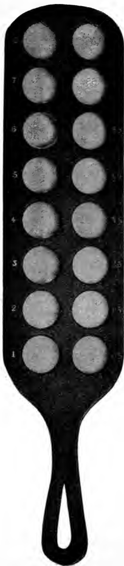
FIG. 51.—Hand frame with lenses for correction with retinoscopy.
