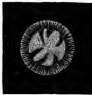
FIG. 22.—Striæ in lens, as appearing with transmitted light.
