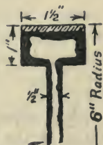
FIG. 15.—Rim of Fly-wheel.
